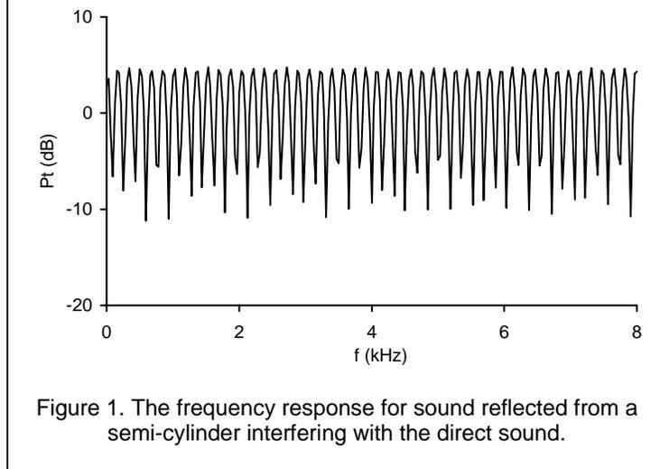
Figure 1. The frequency response for sound reflected from a semi-cylinder interfering with the direct sound.
