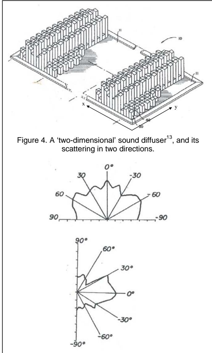
Figure 4. A 'two-dimensional' sound diffuser<sup>13</sup>, and its scattering in two directions.
