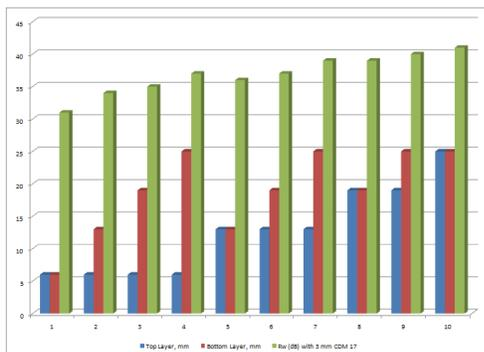
The graph at the left shows the Transmission Loss  $R_w$ (dB) for a variety of plywood thickness/3 mm damping layer/plywood thickness laminations. For example, a constrained layer lamination of 13 mm plywood/3 mm CDM 17/19 mm plywood has an  $R_w$ (dB) = 37.
