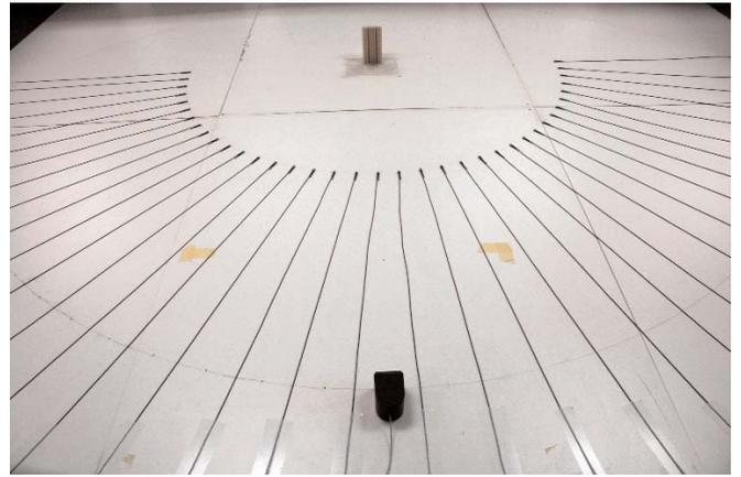
Figure 2. RPG 2D Goniometer with speaker at normal incidence, 37 receiving microphones at 5 degree intervals and a test sample of a QRD. Speaker radius is 2 m and microphone radius is 1 m.
