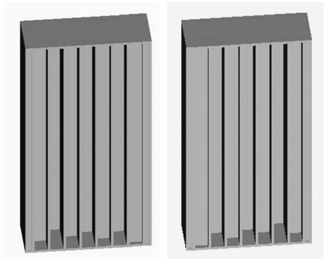
Figure 6: (Left) Binary 0 Unit. (Right) Binary 1 Unit is a mirror image of the binary 0 unit.
