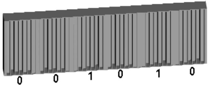
Figure 7. Aperiodic modulation of a single asymmetric shape, which consists of binary 0 units and flipped binary 1 units. Using appropriate optimal binary sequences, an infinite array can be created without introducing any of the problems associated with periodicity.
