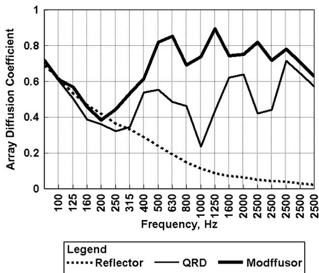
Figure 8. Diffusion coefficient comparison between a traditional QRD and the Modffusor; reveals significant performance improvement, due to the reduction of periodic lobing. A flat panel response of comparable size is also shown to indicate the Modffusor's better low frequency diffusion, as indicated by the onset of diffusion.
