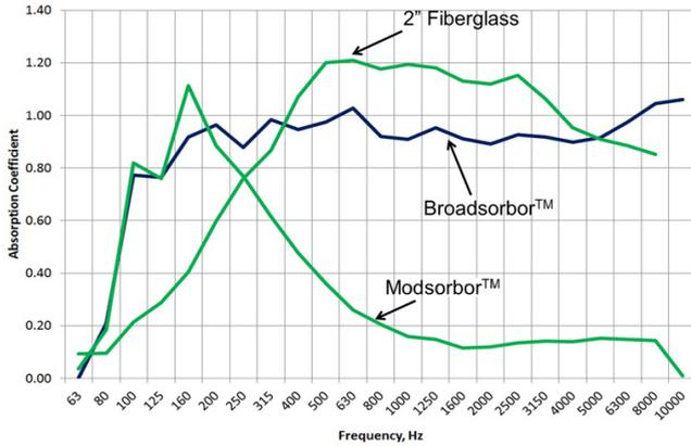
Figure 3. 2" Fiberglass, Broadsorbor and Modsorbor absorption coefficient comparison.
