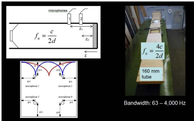
Figure 1. 160 mm square impedance tube using 4 microphones at positions a quarter of the width and height at three positions to determine the surface impedance from 63-4,000 Hz.
