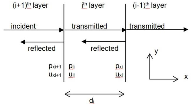
Figure 2. Geometry for propagation of sound through a layer of an acoustic medium.
