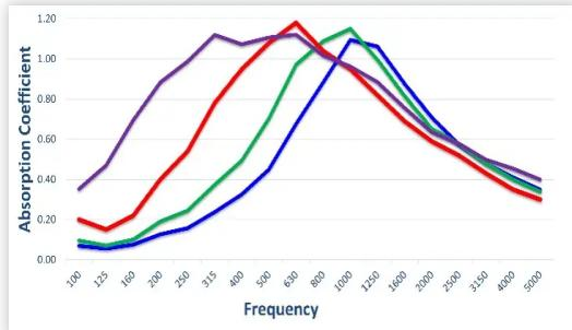
Blue = Beam or Baffle Thickness 3/4" = NRC 0.60
