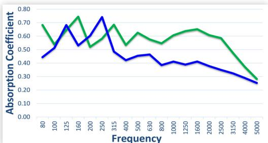
Blue = Single Layer Clearsober® Foil System, 16" airspace behind System to substrate - NRC=0.50, SAA=0.46
